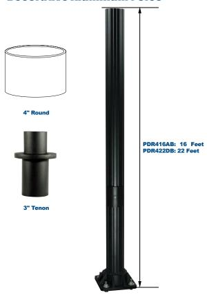
The Jemm Lighting PDR Decorative Round Aluminum poles are built from extruded fluted 11 Gauge aluminum tubing and are offered as direct burial or with a high-strength die cast aluminum base. A pole top plate with a 3" vertical tenon is provided. Typical area lighting applications include retail centers, industrial parks, schools and universities, parks and pedestrian pathways and gathering spaces. Mounting heights to 16 feet can be used based on selected luminaire application.
